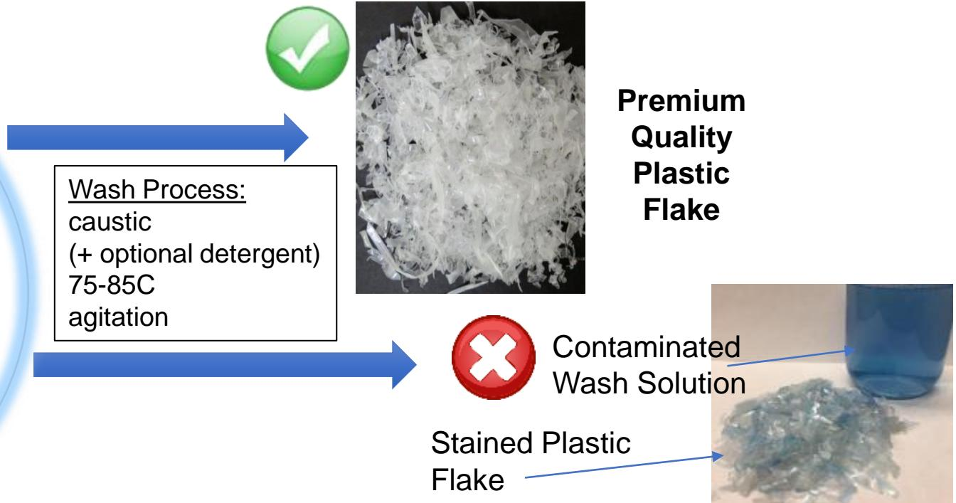
Direct-Printed, Primer-Free Inks That Are Removed and Separated From Recoverable Plastic Substrates Improve Recyclability of Packaging and Enable Industry Certifications. Higher Quality and Quantity of Plastic Flake is Recovered.
